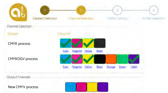
CMYK process dataset and CMYKOGV process dataset are used to build a new CMYV profile.
