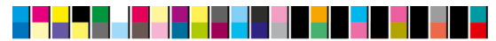
Hydra® control strip for calibration and profiling of a conventional press requires only 48 patches that can be measured in a matter of seconds.
